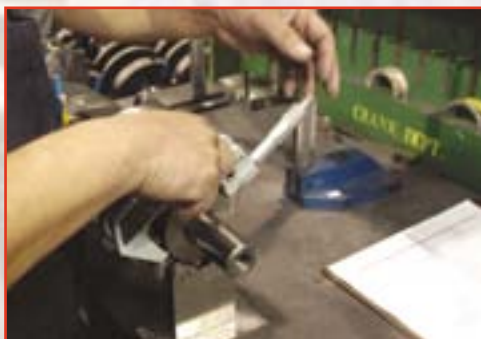
Crankshafts are checked for proper journal dimensions, as well as run-out, taper and rotational eccentricity.
