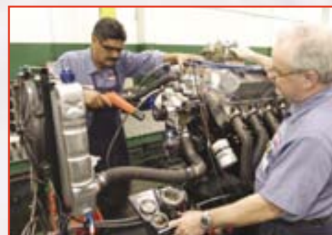
After engines are completely assembled, they are hot-tested (except M6007-XE3M/M-6007-XB3M) to check oil pressure and detect water leaks. The completed engines are run for approximately 20 minutes during this process.
