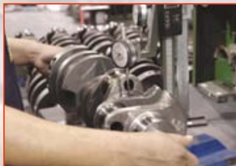
Crankshafts are checked for proper journal dimensions, as well as run-out, taper and rotational eccentricity.
