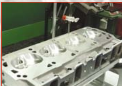
To ensure accuracy of compression ratios of the sealed crate engines (M-6007-D347/M-6007-Z351S), combustion chamber volumes are checked and corrected, if necessary, to achieve proper specifications.
