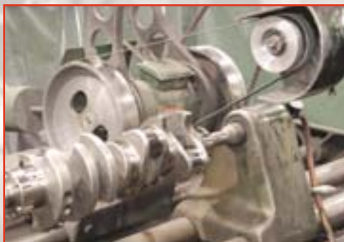
After the crank is polished, the surface is checked to make sure that it meets or exceeds FRPP requirements.
