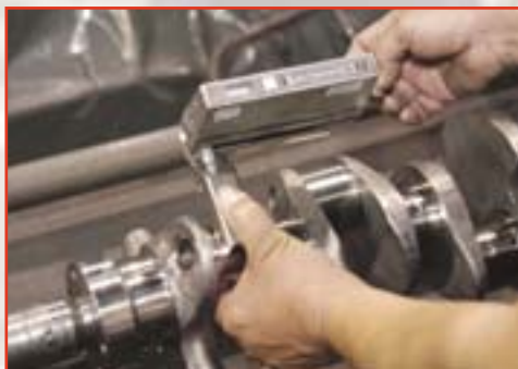
After the crank is polished, the surface is checked to make sure that it meets or exceeds FRPP requirements.
