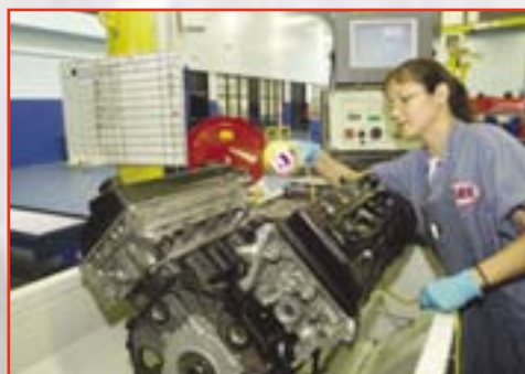
Engine oil has a dye added to it that shows up under black light to reduce the possibility of undetected leaks.
