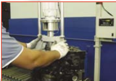
After the short block is completed, the rotating effort is checked to verify proper assembly tolerances.
