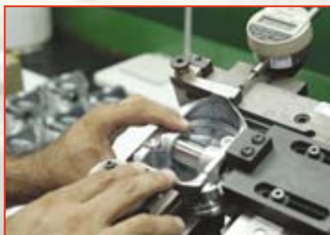
Every piston gets measured and weighed before they are put together in matched sets using strict tolerances.
