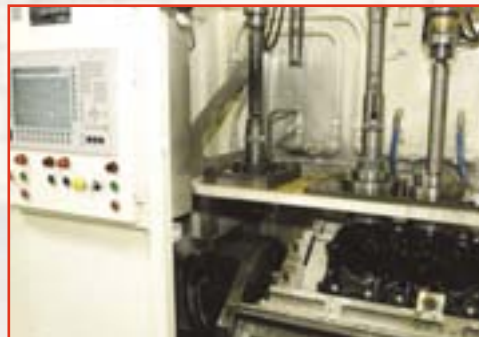
Finish-honing of the cylinder bores is accomplished via a Gehrung CNC hone.
