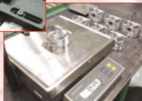
Every piston gets measured and weighed before they are put together in matched sets using strict tolerances.
